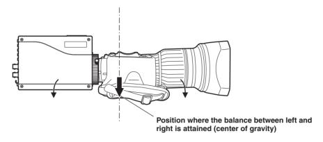
② The less the deviation between the center of gravity position and the head's center of rotation, the more the balance is attained. Check these positions when mounting the pan-tilt head.
